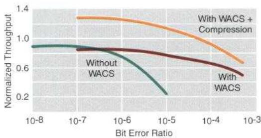
*With the WACS, transmission control protocol/Internet protocol (TCP/IP) transfer performance is significantly improved.*
