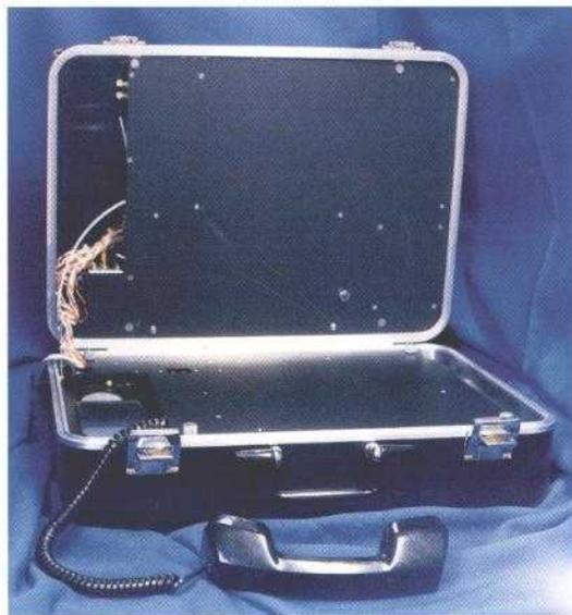
COMSAT Laboratories' portable demonstration C/Ku-band satellite terminal provides voice, data, and fax services from remote sites interconnecting them to the public switched telephone network using available and inexpensive C/Ku-band space segment from DOMSATs or INTELSAT.
