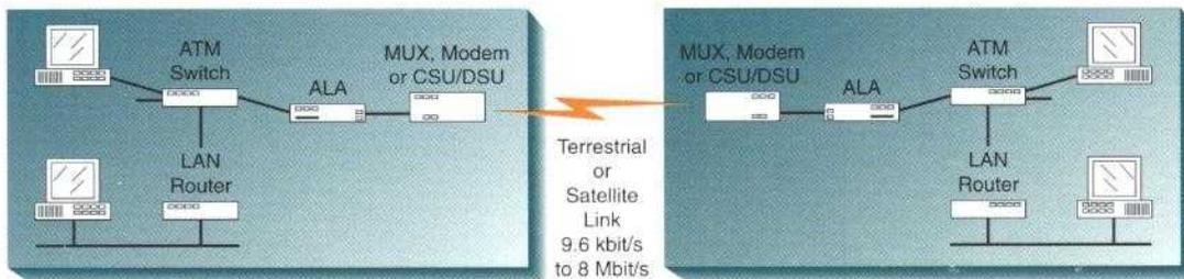
LEFT: The ATM Link Accelerator (ALA) interconnects ATM switches over satellite and wireless links at up to 8 Mbit/s. It offers adaptive coding, data compression, and congestion control to provide fiber-like quality and enhanced throughput for ATM traffic. BELOW: Demonstrated improvement in cell loss ratio performance (TOP) and bandwidth efficiency (BOTTOM) with the ALA.
