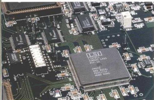
the carrier and clock frequency sources. A COMSAT-patented technique provides programmable data filtering with square-root Nyquist responses and filter rolloffs down to 40 percent.
