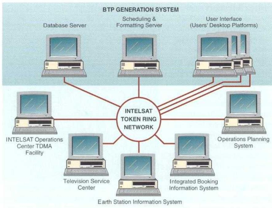
*The BTP generation system will allow INTELSAT planners to generate TDMA BTPs based on station-to-station traffic projections, and to format these plans for distribution via the INTELSAT Operations Center TDMA Facility.*
