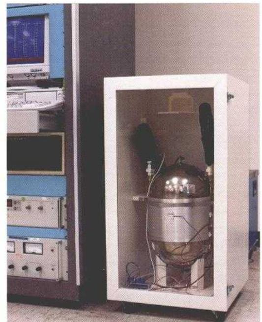
*One of the new lightweight CPV batteries in SSTD's life-test chamber.*
