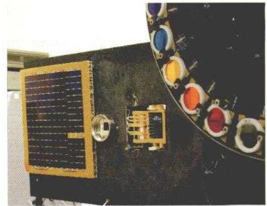
*Solar cells mounted in fixtures on this test plane can be electronically characterized during exposure to a light beam that accurately simulates sunlight level in space at the earth's orbit about the sun. The color filters transmit light only in selected regions of the solar spectrum and are used to determine the solar cell electrical output in these regions.*
