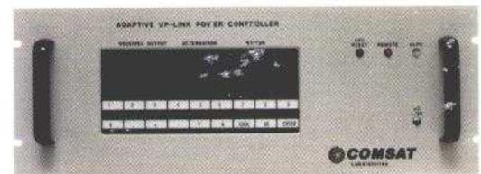
*The prototype ULPC system was built to test and validate the design features of a complete user interface and remote control capability.*
