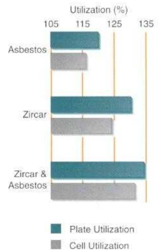
*Destructive physical analysis of Ni-H<sub>2</sub> cells indicates that the coefficient of positive plate active material utilization is higher in cells containing two layers of Zircar™, or one layer of Zircar™ and one layer of fuel-cell-grade asbestos, compared to cells with one layer of asbestos.*
