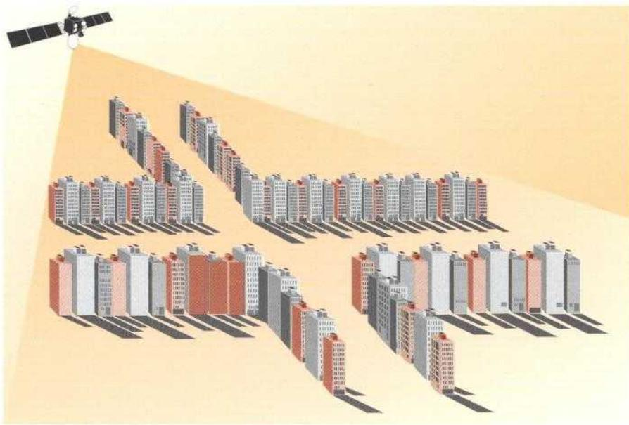
*Computer analysis was used to determine the areas of hypothetical urban landscapes which were blocked from a direct line of sight view of the geosynchronous satellite. Users of handheld terminals in the unshaded areas can always communicate with the satellite, while users in the shaded regions must move to an unshaded region.*
