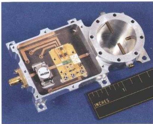
*The 2-W SSPA used for the X-band phased array.*
